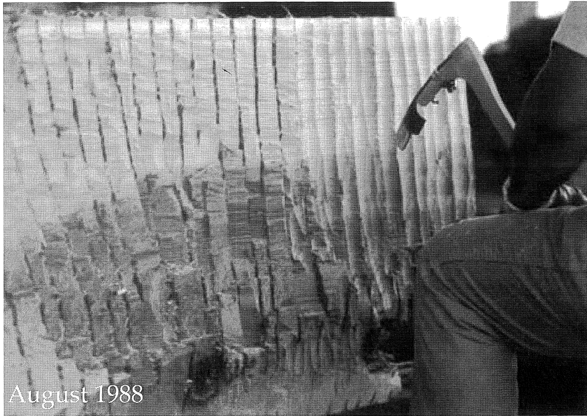
A gutter (elbow) adze is used to shape the right side of the canoe. (Jerry Jones)
