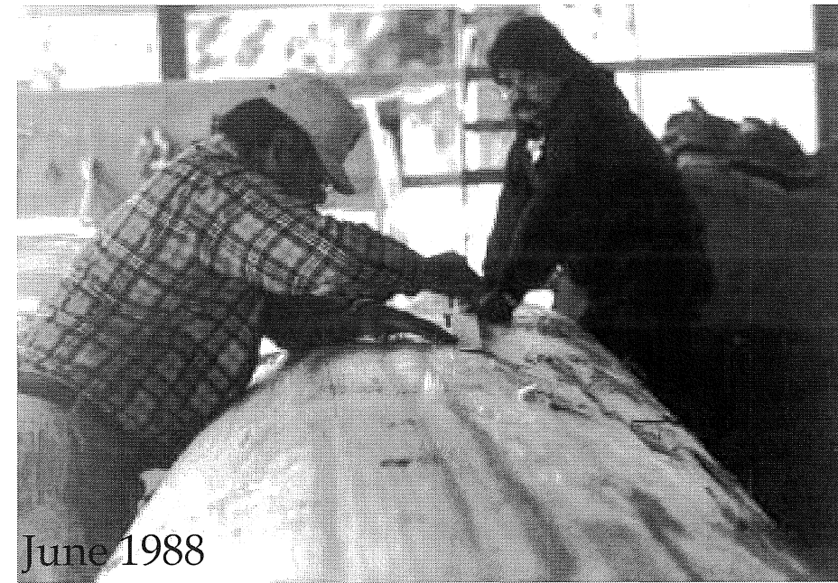
After the top has been flattened, the center line on the bottom is created. (Jerry Jones and Joe Gobin)
